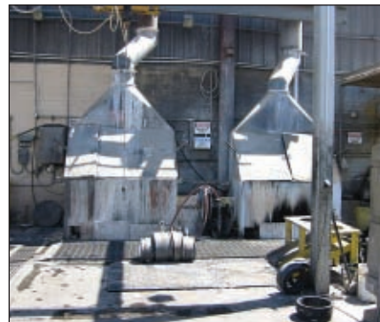
Figure 2. "Before" photo shows old die cleaning tanks. (Wall behind tanks was badly deteriorating.)
